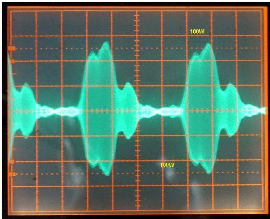
**Test B3b: ALC compression test using 2-tone test signal:** The oscilloscope terminated in  $50\Omega$  is connected to the DUT RF output via a suitable power attenuator. A tone/noise generator program in the connected laptop feeds the 2-tone test signal to the DUT USB port.
